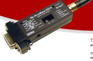
The ProBee-ZS10 is an ZigBee RS232 Serial Adapter with integrated ZigBee core and radio/antenna circuits.
