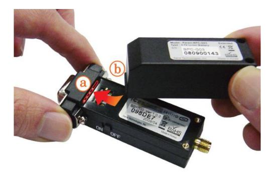
Figure 2-6 Attach the battery pack
