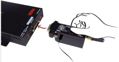
Figure 2-3 Connecting a Serial Device to Parani-SD1000
