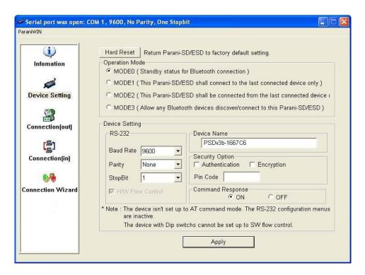
Figure 3-6 Device Setting Window
