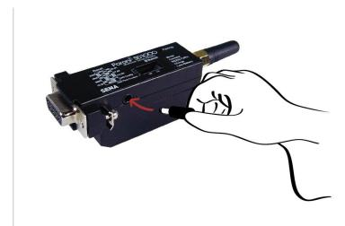
Figure 2-2 Connecting Power to Parani-SD1000
